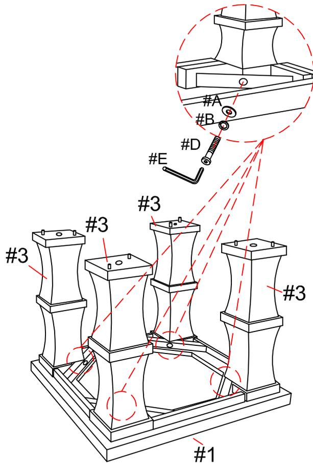
Prepare 4 bolts assembly by inserting locker washer (#B), then flat washer (#A) to the bolts (#D). Secure legs (#3) to table top (#1) with bolts (#D) using the Allen wrench (#E).
