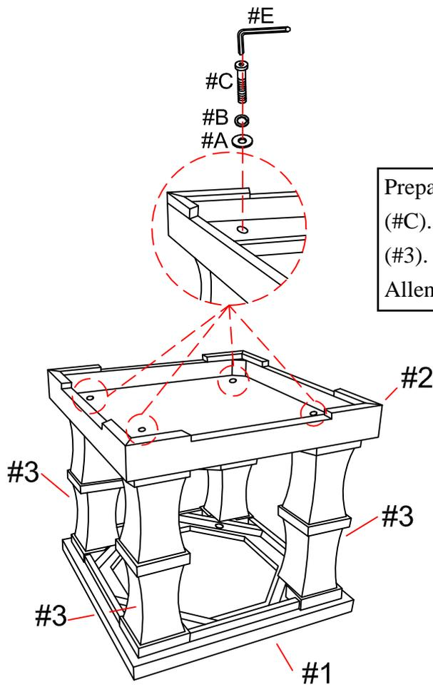
Prepare same 4 bolts assembly with bolts (#C). Align table bottom (#2) to the legs (#3). Secure with bolts (#C) by using an Allen wrench (#E).
