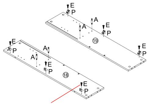
It is recommended to use an electric drill to assist installation.
