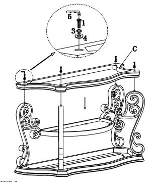
STEP 3: Attach Bottom Panel (C) to Legs (E) by using Allen Key M4 (5), Allen Bolt 1/4" x50mm (1), Spring Washer 1/4" (3), Flat Washer 1/4" (4)
