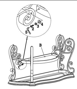
STEP 2: Attach Shelf (B) to Legs( E) by using Allen Key M4 (5), Allen Bolt 1/4"x28mm (2), Spring Washer 1/4" (3), Flat Washer 1/4" (4)
