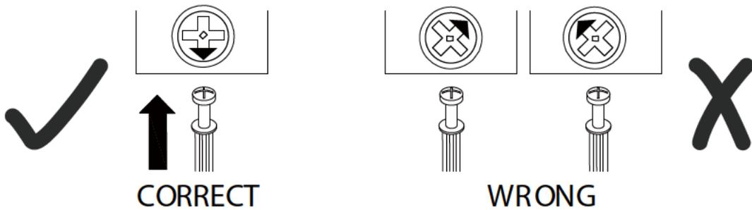
Quick fit head should be in the centre of the cam lock when the two panels are rejoined. Cam lock should be inserted before quick fit.
