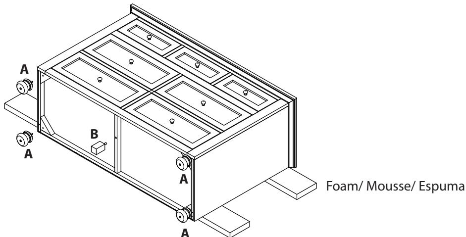
Place Dresser on some foam as shown. Then attach 4 Round Legs (A) into 4 holes at corners under Dresser, and Support leg (B) into the hole of middle Dresser.
