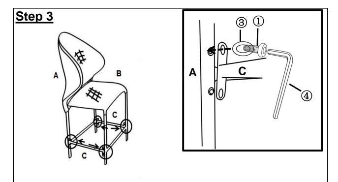
Attach Rail(C) between Backrest(A) and Front Legs of Seat Base(B), using Bolt(①) and Washer(③) with Allen Key(④).
