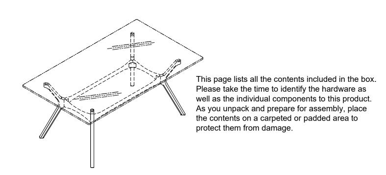
Attached four Legs(B) to the Leg Frame(C). Use Bolt(D) Lock Washer(F) and Flat Washer(G) on holes of Leg Frame(C). Turn the Allen Key(H) in Allen Bolt(D).
