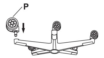
Turn the Base upside down, press the Casters(**P**) into the holes at the end of each Leg.
