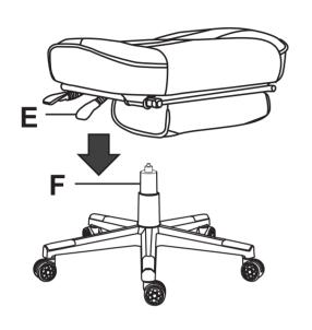
Position the assembled chair upright with the Seat Mechanism(**E**) facing down. Insert the Gas Lift(**F**) into the center hole of the Seat Mechanism(**E**) and press down until fully engaged.
