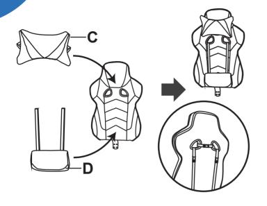
Connect the elastic rope of the Headrest(**C**) and the Lumbar Backrest(**D**) through the holes of the chair back respectively.
