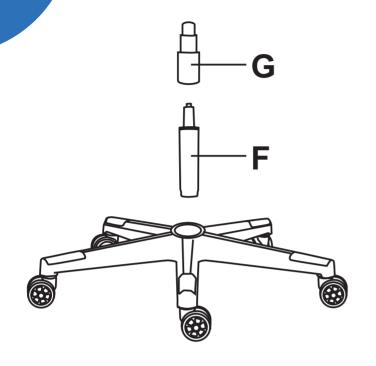
Then insert the Gas Lift(**F**) into the center hole of the Base. The Telescope Cover(**G**) should be placed over the Gas Lift.
