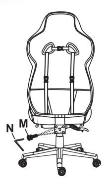
Align the pre-drilled holes on the back connector. Then fix it with the Bolts(M) and Wrench(N).
