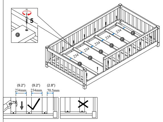
Note: Do not lock the screws of the bed slats to the outermost edge of the bed slats, you need to leave a certain space at the edges, otherwise it will cause the board to break. Do not lock the bed slats on the edge of the wood, please hold firmly before screwing, hold it in place with one hand, then lock the screw.
