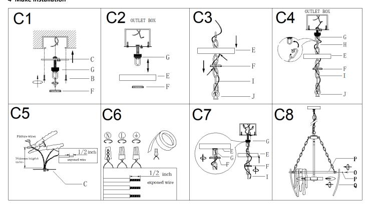
Step C1: Remove the collar ring (F) from collar loop(G). Attach the single bar (C) to outlet box with mounting screws(B).
