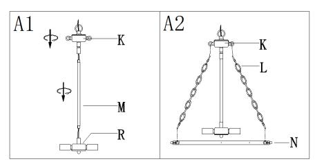
Step A1: Slip stem (M) over the wires and then thread it into the top of lower fixture loop assembly (R). Slip upper fixture loop assembly (K) over wires and then thread it onto the top of stem (M).
