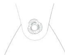
Snap Rivet TIP facing INSIDE of Lamp
