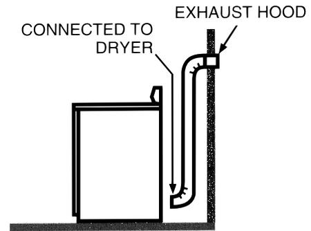
3. Clean exhaust duct from end where dryer is connected to the exhaust hood using:
