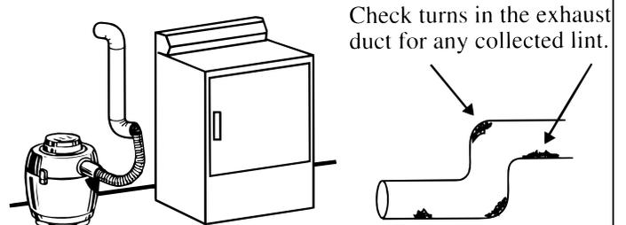
4. Inspect exhaust hood. To minimize resistance to the exhaust air flow:
