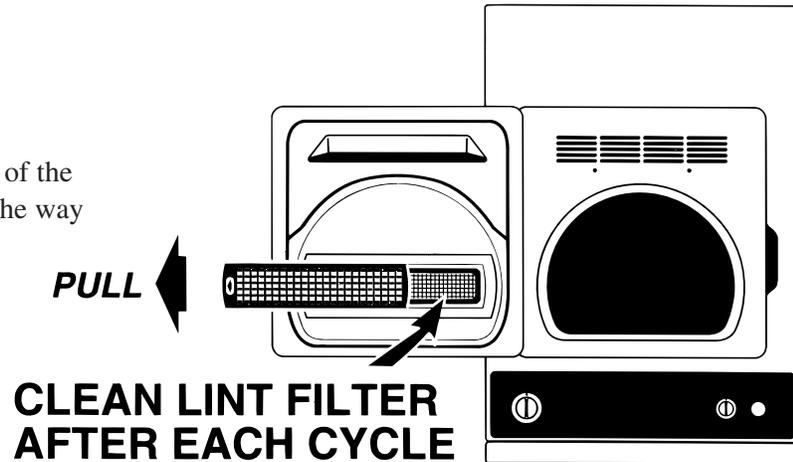
*Do not operate the dryer without the grid in place.*
