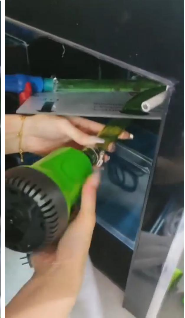
Another pipe goes through the hole in the cover first, and then connects the pump
