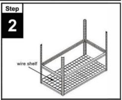
Start by adding a wire shelf to the level previously built, then continue working by adding the second level using two (2) beams and two (2) braces in the post slots of your desired location. Again place the rivets of the beams and braces into the post slots with the shelf ledge facing up and tap lightly to seat the rivets.
