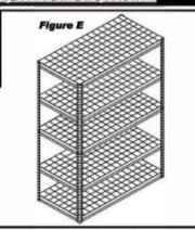
Add a wire shelf to the previously built level, then continue by adding the fourth and fifth level to the unit using two (2) beams and two (2) braces per level. Tap lightly to properly seat the rivets and add the final wood shelves to the unit (see figure E).
