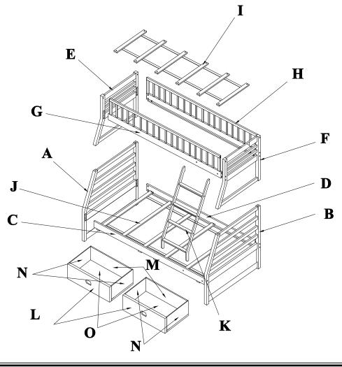
STEP 1: LOWER (Left + Right) HEADBOARD & LOWER (Front + Back) SIDE RAIL ASSEMBLY
