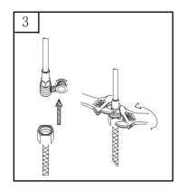
Attach rubber washer and metal washer onto copper tubes. Screw metal threaded rods onto faucet body.
