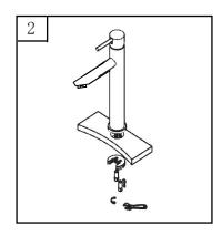
2.Screw cold/hot copper tube onto faucet body.
