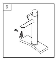
5. After installing faucet, remove aerator and turn on water to remove any left over debris. Re-assmble aerator.
