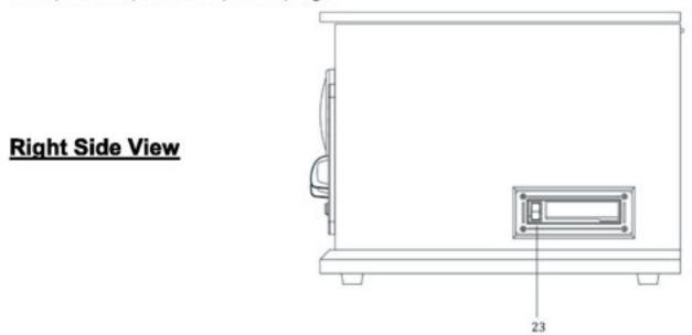
23. CASSETTE FF & EJECT Press halfway to fast forward, press all the way to end and eject the tape.
