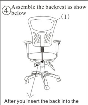
After you insert the back into the mechanism and adjust to desired height, turn the button counter-clockwise until it is screwed in tightly.
