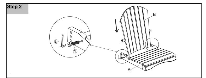
Attach Backrest Panel(B) to Seat Panel(A) using Screws(1) with Allen Key(5) as shown above.
