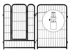
Please install the two "plastic connected silencers" between the adjacent holes to reduce friction and noise.
