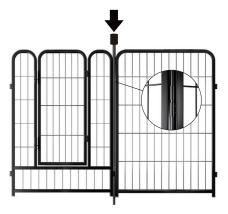
Insert the cylindricity up-sided stick into the holes of the two connected pieces.
