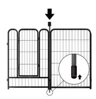
Insert the cylindricity up-sided stick into the holes of the two connected pieces. Please install the "floor protectors" to the end of "cylindricity up-sided insertion" when Indoor Use.
