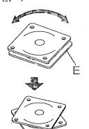
Rotate Seat Swivel (E) as shown to expose all of the bolt holes
