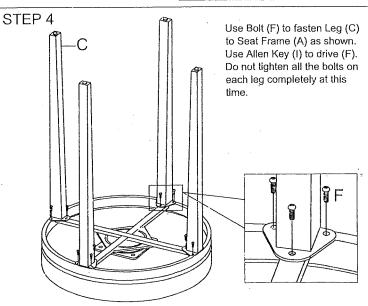
Do not tighten all the bolts completely at this time. See STEP 5.
