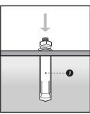
Fasten nut with socket wrench to fully secure expansion bolt to concrete.
