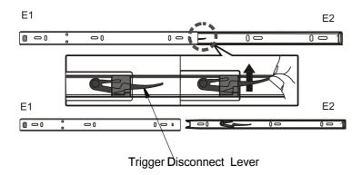
To install Drawer Slide, the Drawer Slide Runner (E2) needs to be detached or separated from the Drawer Slide Rail/Track (E1).
