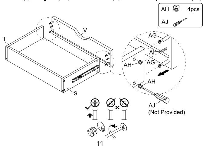
Assemble the pre-assembled drawer box by using Slide Rail (W) into the pre-assembled drawer frame. Move Slide ball spacers the front. Hold drawer horizontally, and slide runners into ball spacers.
