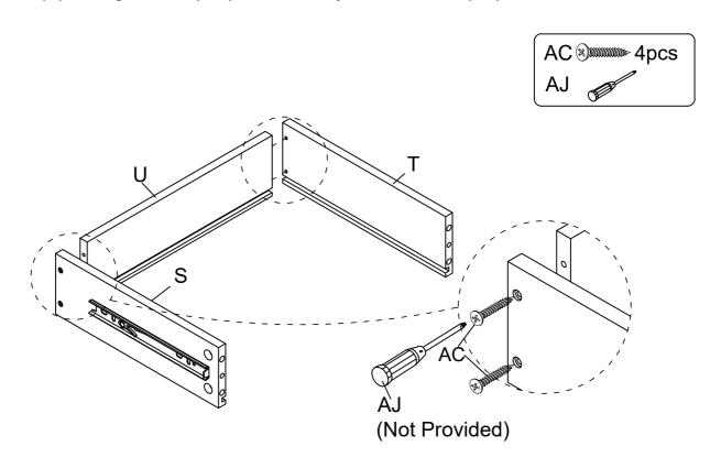
Assemble Drawer Board - Bottom (R) to Drawer Left Panel (S), Drawer Right Panel (T) & Drawer Back Panel (U).
