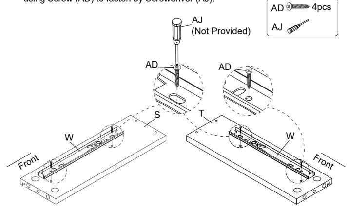
Assemble Drawer Back Panel (U) to Drawer Left Panel (S) & Drawer Right Panel (T), using Screw (AC) to fasten by Screwdriver (AJ).
