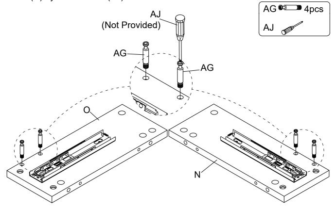
Assemble Drawer Side Board - LSF (O) & Drawer Side Board - RSF (N) to Support Panel (Q), using Nut (AH) to lock with Bolt (AG), then fasten by Screwdriver (AJ).
