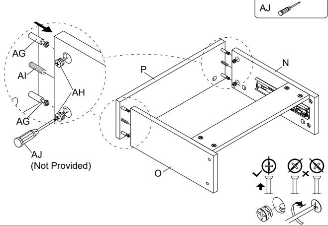
8 Assemble Bolt (AG) & Wood Dowel (AI) to Drawer Board - Top (M) by Screwdriver (AJ).
