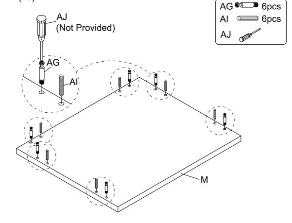
Assemble Drawer Board - Top (M) to Drawer Side Panel - LSF (O), Drawer Side Panel - RSF (N) & Drawer Board - Back (P), using Nut (AH) to lock with Bolt (AG), then fasten by Screwdriver (AJ).
