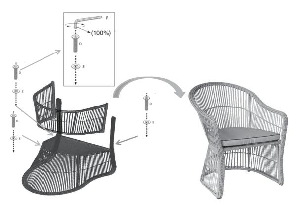
Attach runner (B) to chair (A) and secure by using screws (D+E).
