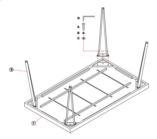
NOTE: DO NOT TIGHTEN ALL THE BOLTS UNTIL THEY ARE INSTALLED IN CORRESPONDING HOLES!
