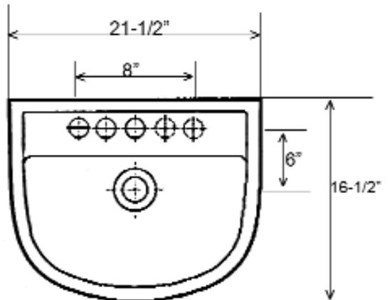
Dimensions of fixture are nominal and may vary within the range of tolerances established by ANSI Standard A112.19.2-2013. Dimensions and specifications subject to change without notice.
