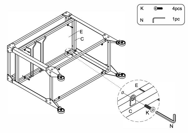
Assemble bottom panel (F) to bottom frame (D) respectively with bolt (K) as shown in drawing. Then tighten up with allen wrench (N).
