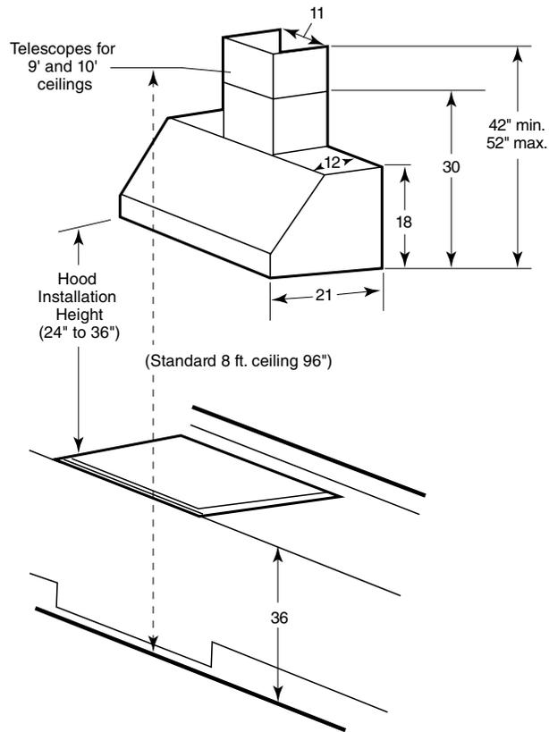
Installed above a range (shown with optional chimney kit)
