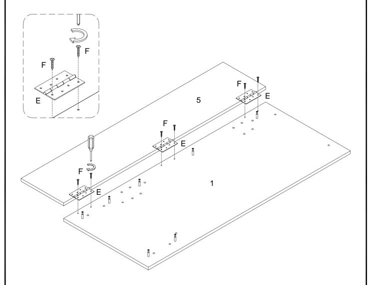
Using screw (F) attach hinge (E) into part (1) with Philips head screwdriver as per diagram .
