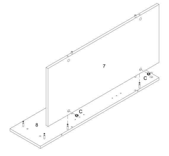
Using cam lock (C) secure part (7) into part (8) with Philips head screwdriver.
