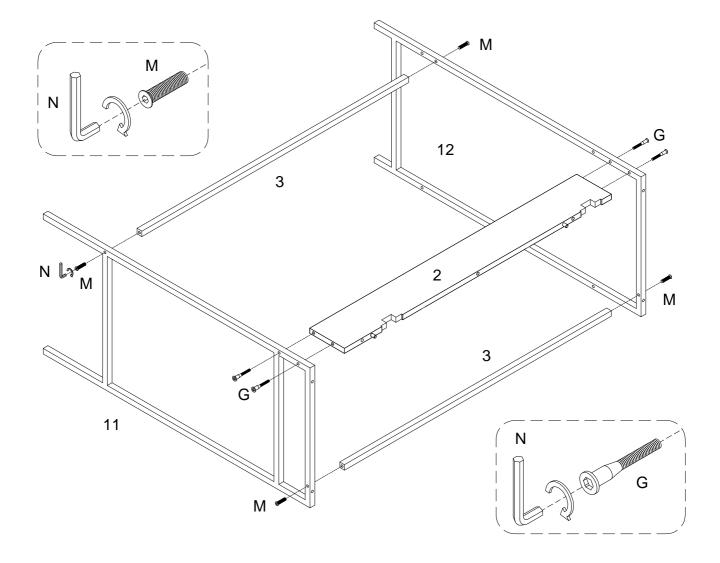
Using bolt (M) attach parts (3) into parts (11,12) ,use bolt (G) attach part (2) into parts (11,12) with hex key (N) as per diagram.
