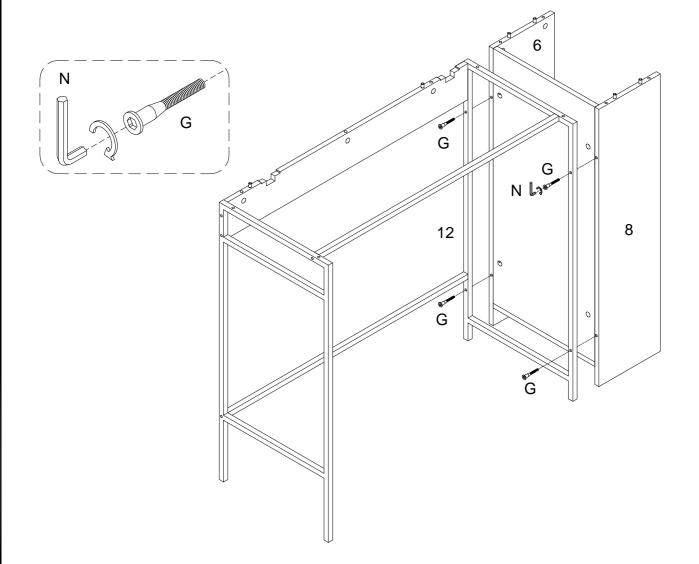
Using bolt (G) attach part (12) into parts (6,8) with hex key (N) .
