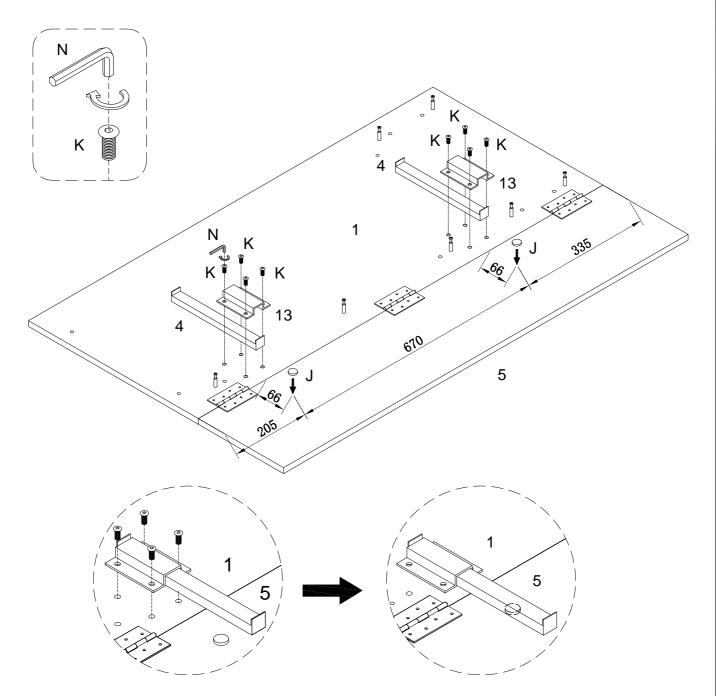
Attach rubber pad (J) on part (5) as the diagram .please keep the rubber (J) and part (4) in the same line .ln this way when you pull out the leaf support (4).it could be on the rubber pad (J). Using part (13) cover part (4).then use bolt (K) secure part (13) to part (1) with hex key (N) as per diagram.
