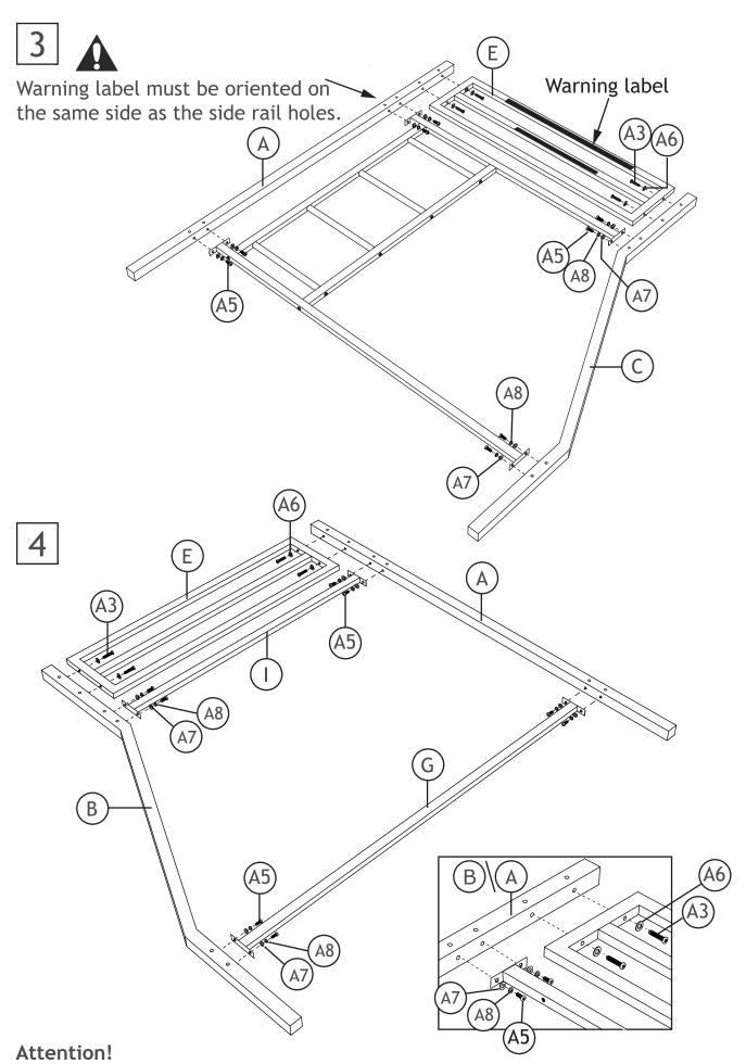
Do not tighten up the screws until all the screws are aligned with the holes.
