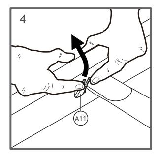
4. Press tight the upper part of clamp to fix its position.
