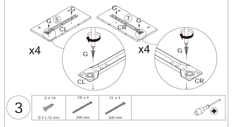
Fix rail(CL) to plate 6 with screw(G) at first. **Flip to back,** fix rail(CR) as shown.
