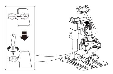
Use the screwdriver 4 to tighten the 2 screws just removed and put the cap on.
