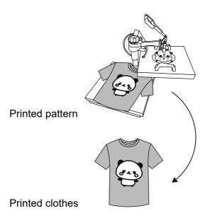
Turn off the power and pull out the mat. It is recommended to wear heat-resistant gloves when removing clothes or remove them after 2-3 minutes. Be careful of hot heat.
