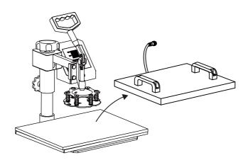
Rotate the heat transfer board to the side.
