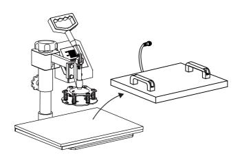
Rotate the heat transfer board to the side.
