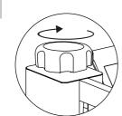
Turn this adjustment switch to adjust the pressure.
