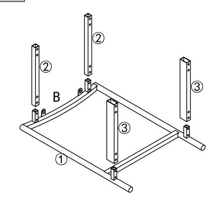
Attach 2 x parts (2) and 2 x parts (3) to part (1).
