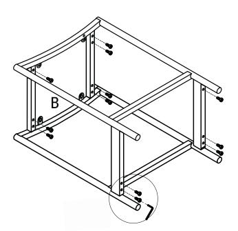
Tighten the 16x bolts (B) completely until all bolts are lined up and inserted into holes.
