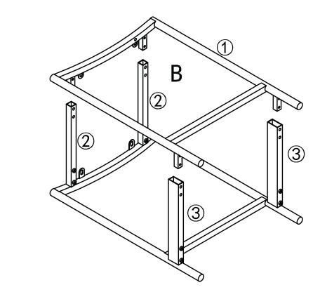
Attach the other part (1) to the parts (2) and parts (3).
