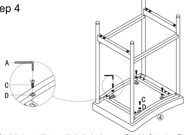
Attach the top part (4) to assembled unit using 4 x screws (C) and 4 x flat washers (D) with Allen Key (A).
