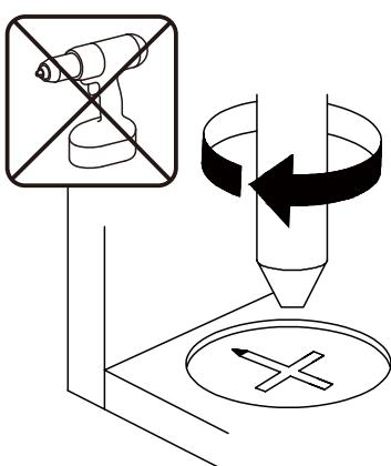
**EN**\_Turn cam lock clockwise to tighten.
