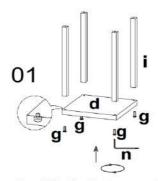
Step1:Fix the bottom panel and the wooden pole firmly with the hex screws.Please note that the sink screw holes are facing down.
