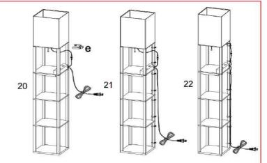
Step 20-22: Clip the wire clamps on the lamp poles and clip the wire into the clamps well.
