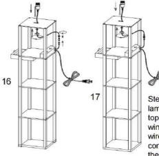
Step16-17: Fix the lamp holder on the top panel with the wing nut, fasten the wires with the selfcontained nut from the USB box.
