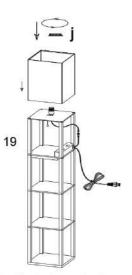
Step 19: Fix the lampshade on the lamp holder with the lamp nut. (Unscrew the nut from the holder firstly)
