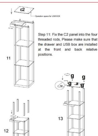
Step 12: Tighten the wooden poles and fix them on the fourth panel.
