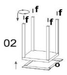
Step 2: Stick the EVA cushion on the bottom of the bottom panel. Rotate the threaded rods and fix them to the tops of the wooden poles.
