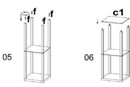
Step 5-6: Tighten the wooden poles and fix them on the second panel, then place the third panel on the four threaded screws.
