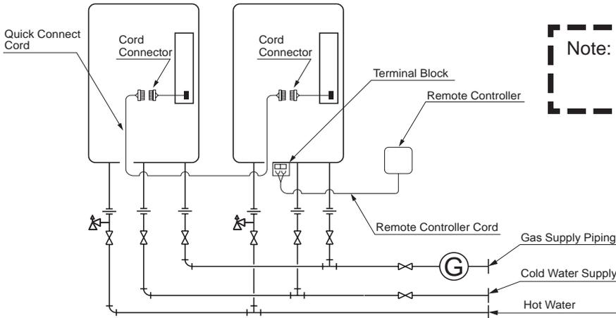
Note: Connect the remote controller to only one of the units.
