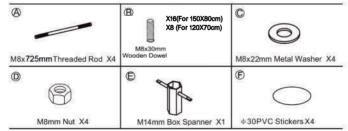
**NOTE:** The quantities above are the correct amount to complete the assembly. In some cases more fittings may be supplied than are required.
