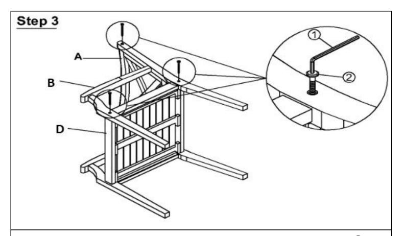
Attach Right Leg Panel (B) to Seat Panel (D) and Backrest Panel (A) by using 3 Screws ((2)) with Allen Key ((1)).
