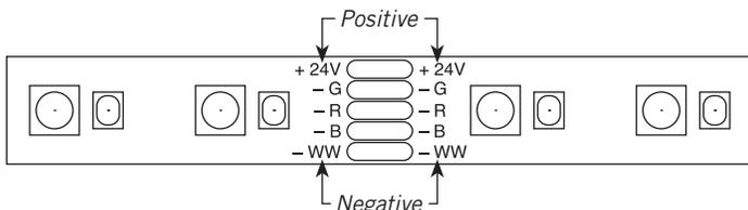
**NOTE:** Be sure all 24-volt connections are secure and protected from electrical shorting. Options include electrical tape, small wire nuts, crimp connectors, etc.
