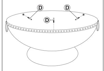
Hand-tighten three M8x25mm Grub Screws (D) to the inside rim of Fire Bowl (B).
