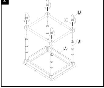
$\label{eq:continuous} \frac{\textbf{Step 1}}{\textbf{Insert Bolted end of Post (B) into hole on bottom of Table Top}}$ (A). Twist 4 Posts clockwise until tight.
