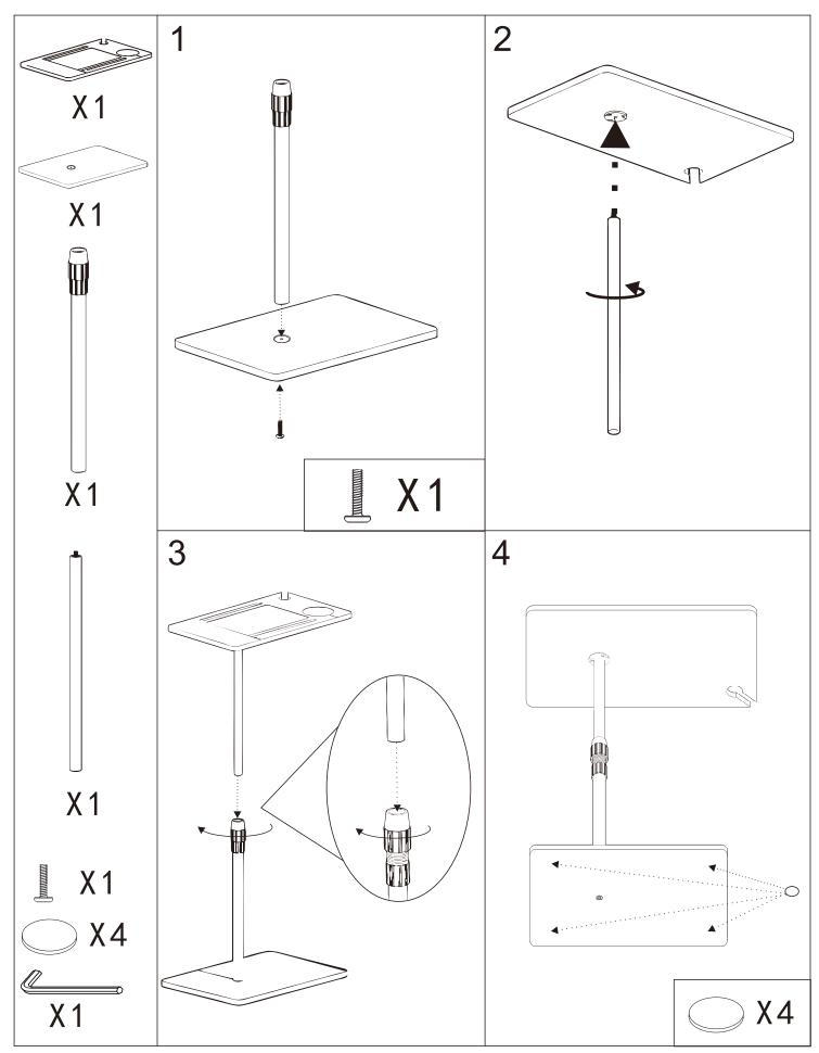
Step 3 of the manual: The plastic positioning can rotate 360 degrees, The height can be freely adjusted, and the overall height can be adjusted to 60cm.
