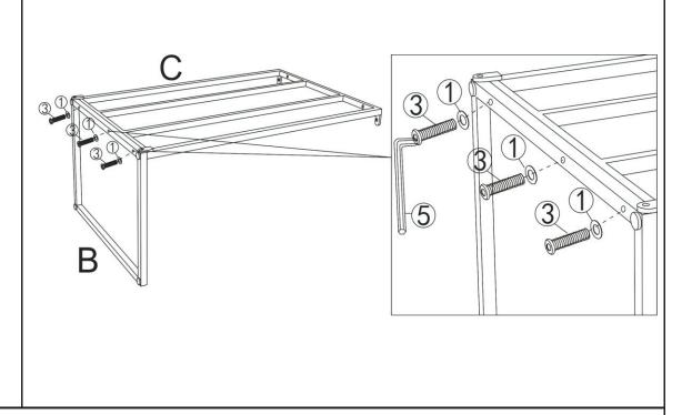
Align the mounting positions on the Support Bar(B) and the Leg(C), Then attach Leg(C) to Support Bar(B) using Washer(1) and Bolt(3) with Allen Wrench(5) as shown.
