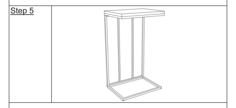
In a sequential manner, drive in and fully tighten all Bolts at all joints. Thereafter, turn the Table right side up. Your Table is now ready to for use.
