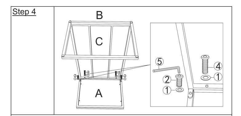
Align the mounting positions on the Table Top(A) and the Leg(C), Attach Leg(C) to Table Top(A) using Washer(1) and Bolt(4) with Allen Wrench(5) as shown.
