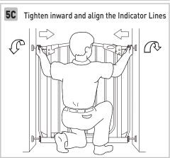
6. Tighten the Tension Knobs until the two Indicator Lines, located on the Upper Locking Set and on the Right Upper Corner, align horizontally (6A).
