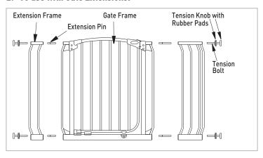
Insert Extension pins into the holes on the outside of the Gate Frame (2A / 2B).
