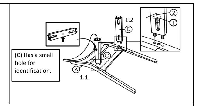
**1.1)** Insert the Side Stretcher(C) and Side Stretcher(D) into the Chair Back(A) as shown.
