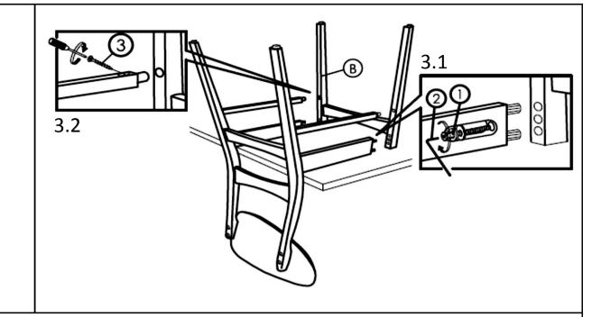
Insert Front Leg(B) onto the Side Stretchers and Side Rails as shown.
