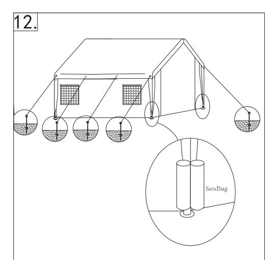
Fixed and tightened the 8pcs ropes ,and then the 4pcs sandbags filled with sand or soil tied in the four corners of the leg tubes.
