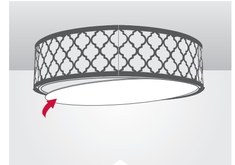
STEP 6: Install the diffuser into the drum.
