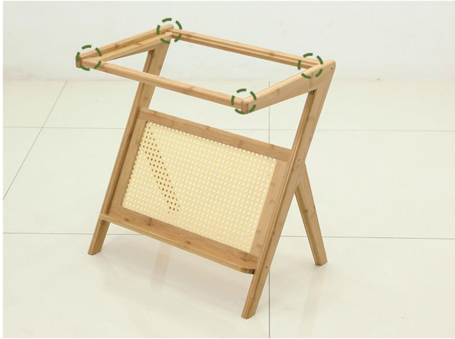
5.Remove spacers and attach them to the four corners of the frame
