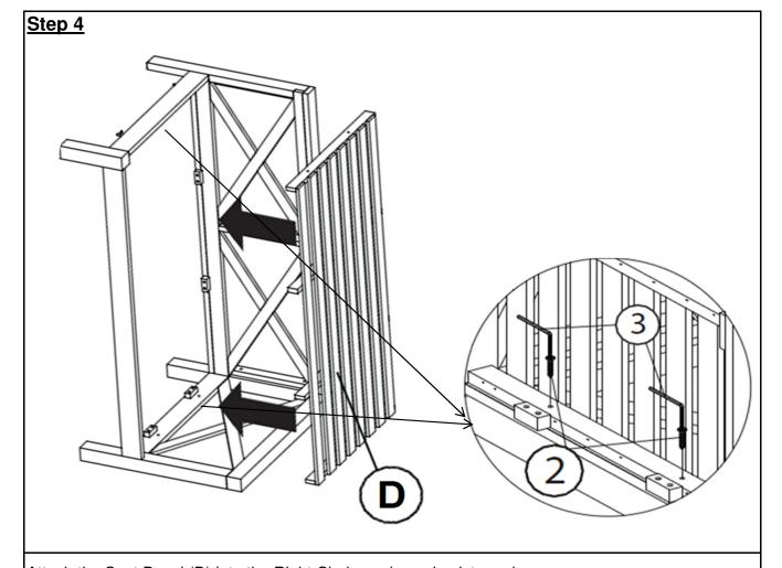
Attach the Seat Panel (D) into the Right Chair as shown in picture above. Affix Seat Panel (D) with Corner Chair by using Screws (②) and Allen Key (③).
